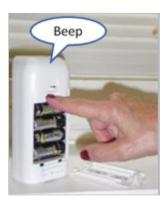
Remove the battery cover at the back of the AbiSensor.
