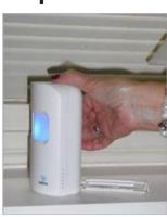
Once the AbiSensor is ON, press the **black button** again. The sensor will light up blue and enter Bluetooth mode.
