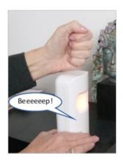
Continuously tap or shake the AbiSensor firmly up to 10 times (to activate the vibration sensor) and wait up to 30 seconds until it beeps and the light turns red.
